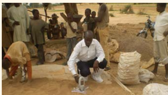
Dr. Suleiman Haladu - a Resident of the Nigeria Field Epidemiology and Laboratory Training Program (NFELTP) determining lead soil contamination levels using XFR machine in Zamfara State, Nigeria
